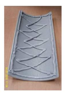
The wearpad area should be solvent cleaned to remove dust, debris and grease. Apply the FibaBond using a caulking gun ensuring a continuous seal at the edges of the wearpad and then apply enough in the middle of the pad to ensure a secure bond to the pipe. The wearpad can then be positioned on the pipe.
